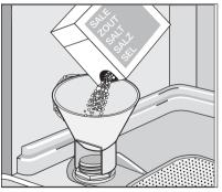
**1** The salt indicator light on the control panel can remain illuminated for 2-6 hours after the salt has been replenished, assuming the dishwasher remains switched on. If you are using salts that take longer to dissolve then this can take longer. The function of the machine is not affected.
